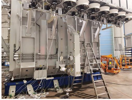
Figure 9. Transformer with the acoustic sensors on the tank wall. Other sensors are also placed on top and at the other side of the transformer
