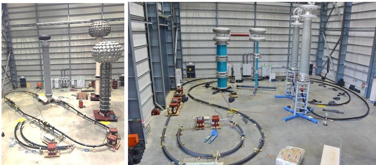
Figure 19. links: HVDC 525 kV Type Test [18], rechts: 525kV HVDC PQ test, 1 Jahr, 100m Kabel, [19]
