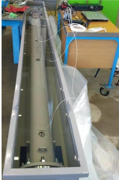
*Figure 5: Impedance tube for use in transformer oil.*
