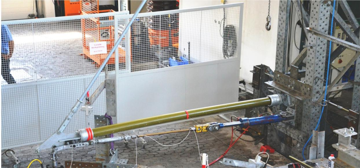
These tests were very useful as they revealed some weaknesses in the original design of some pieces (hinge e.g.) as well as connection parts.
