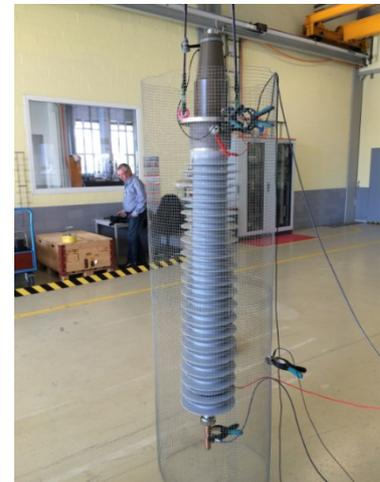
Figure 13: grounded Faraday cage to isolate measurement from interference (ABB)
