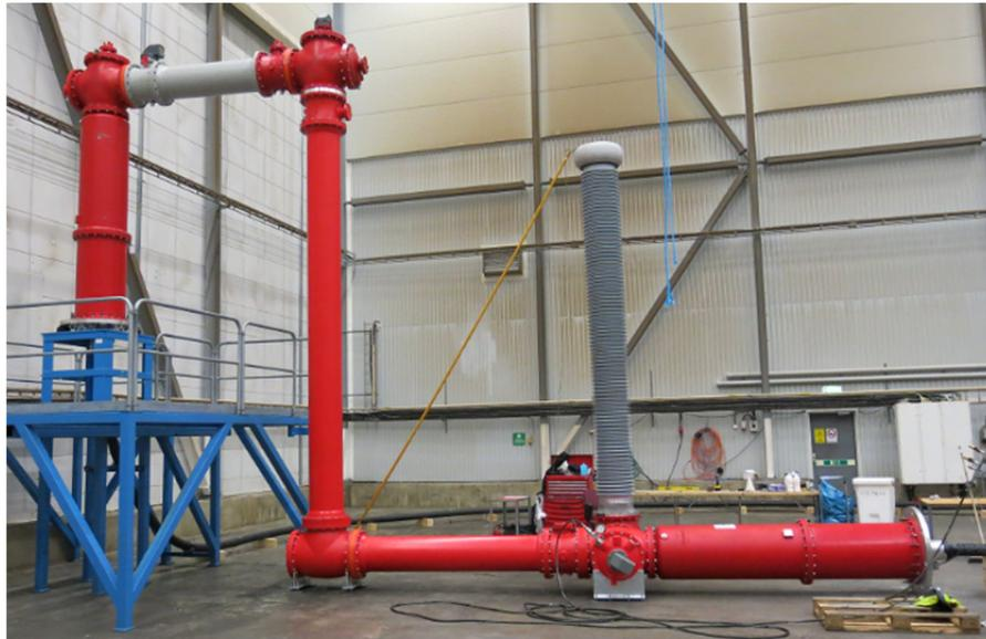
Figure 7 Test set-up for a vertical (left) and horizontal (right) HVDC GIS termination including a cable loop.
