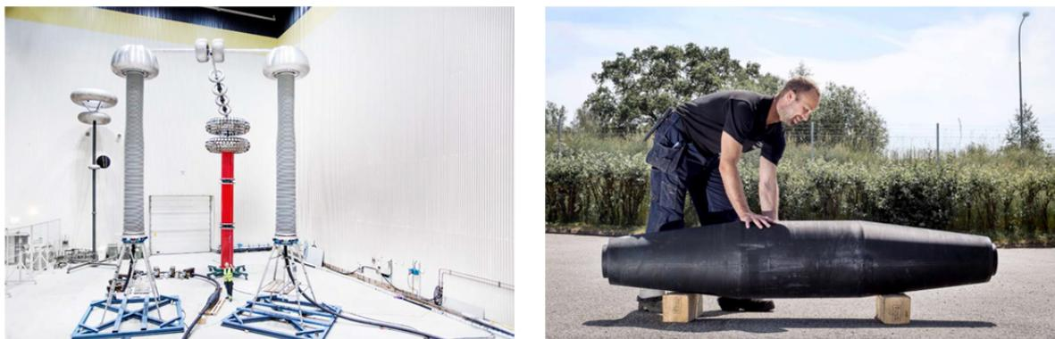
Figure 10 Type testing of the 525kV extruded HVDC cable system (left) and a 525 kV rubber body of a pre-fabricated joint (right)
