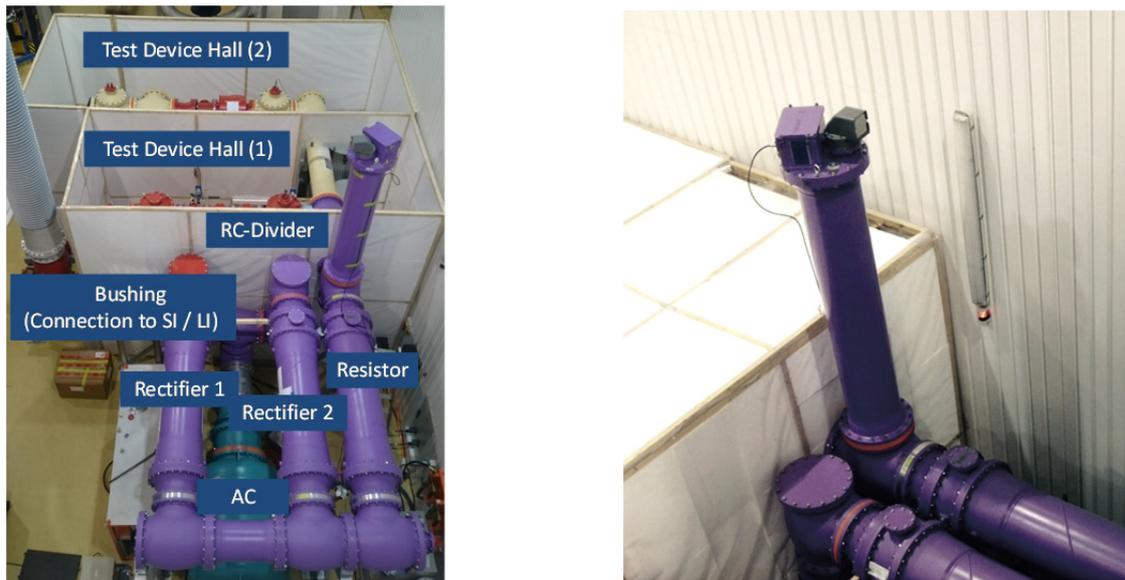
*Figure 5 DC insulation system: test set-up for testing of different insulators in parallel (roof of test device halls were removed for photos only) and RC voltage transformer (right)*
