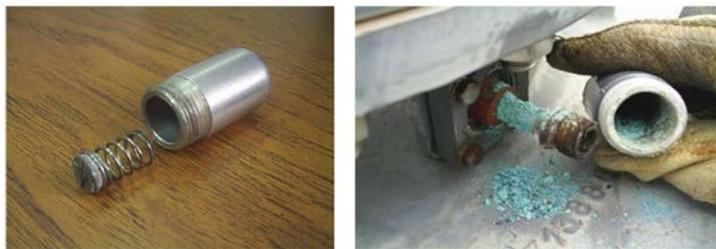
*Figure 6a: Examples of corroded sensor taps which can result in destruction of the bushing itself ('Diagnostic Experience on HV Bushings Retired from Service', M. Guzman, CFE, 2015 INMR World Congress); the utility decided to abandon on-line bushing measurements*
