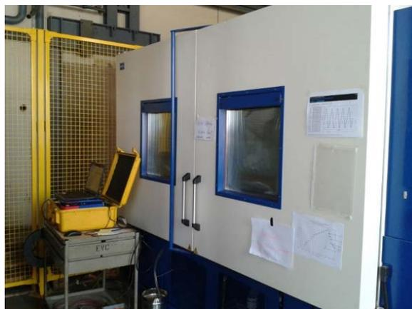
Figure 8: DFR measurement in climate chamber (ABB MICAFIL)
