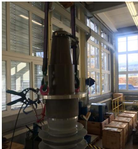
Figure 12: shielding on oil side (ABB MICAFIL)
