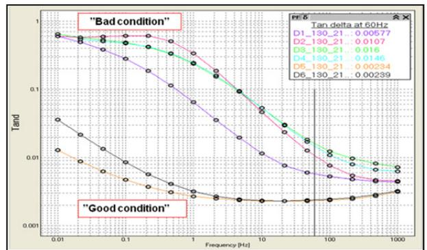
Figure 8. Right: Tan delta vs frequency measured at 0.13 kV and ambient temperature
