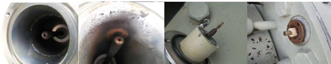
*Figure 6b: Examples of failed bushings due to corroded on-line measurement sensors (bushings serviced/replaced by ABB TRES, Germany)*
