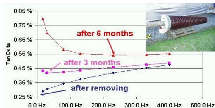
Figure 3: Dielectric Response of a RIP bushing exposed to moisture
