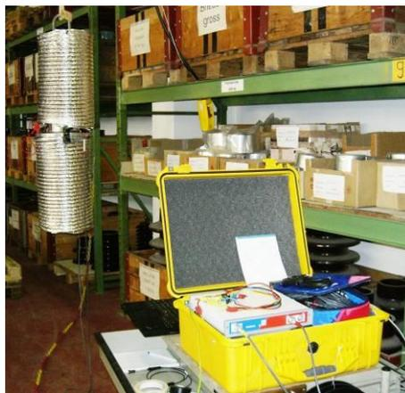
Figure 10: Combined FDS-PDC measurement on a RIP bushing with an Aluminum shield for interference protection
