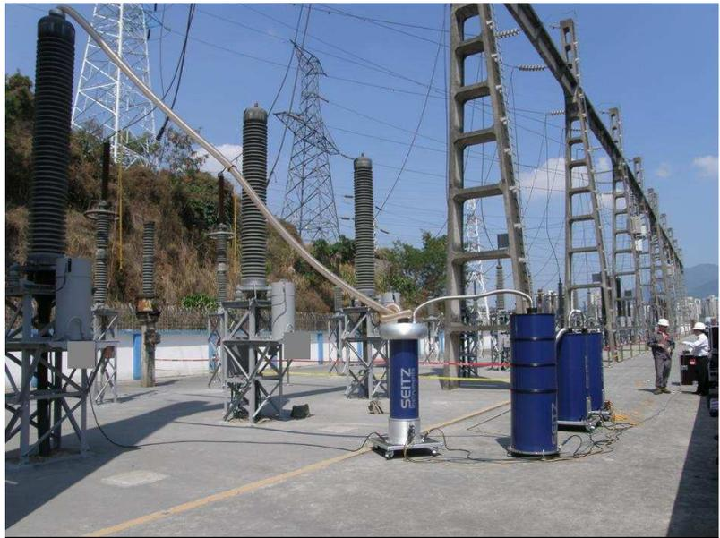
Figure 3. Example of modern monitored on-site testing and diagnosis by partial discharges and dissipation factor measurements using sinusoidal damped AC voltages: maintenance test of a 220 kV cable circuit.
