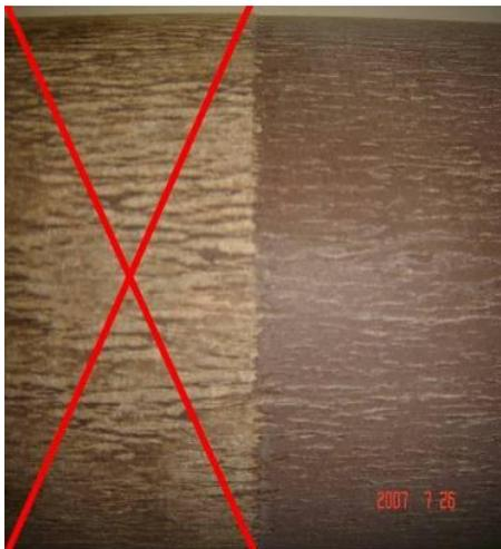
Figure 15: Resin surface damaged by water
