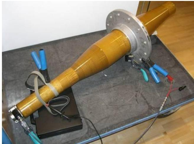
Figure 16: Wrongly stored RBP bushing
