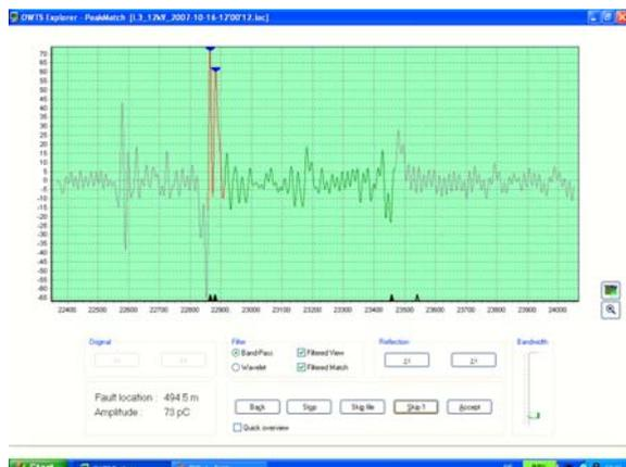
Figure 4: TDR trace of PD fault located 15 m to far end
