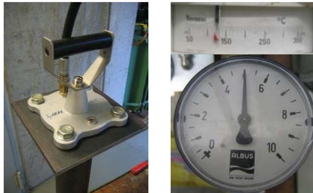
Fig. 4: Picture of leakage test; left) UHF PD probe attached to a test vessel, right) Measured temperature and pressure
