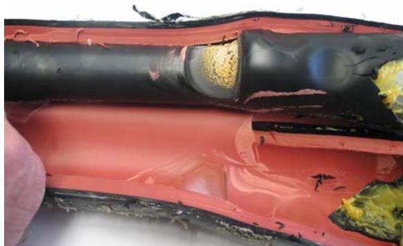
Figure 13: Wrong connector size causes PD in gaps between field stress and insulation components of joints
