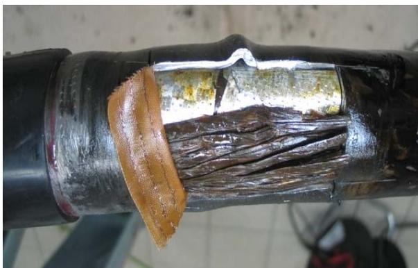
Figure 10: Mechanical damage due to strong bending causes PD in PILC insulation
