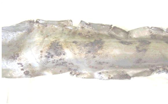
Figure 11: Lead sheath corrosion on PILC causes mass leakage and PD in dry areas of the paper insulation
