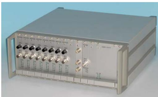
Fig. 8. multichannel acoustic PD measurement instrument (here LDA-6)
