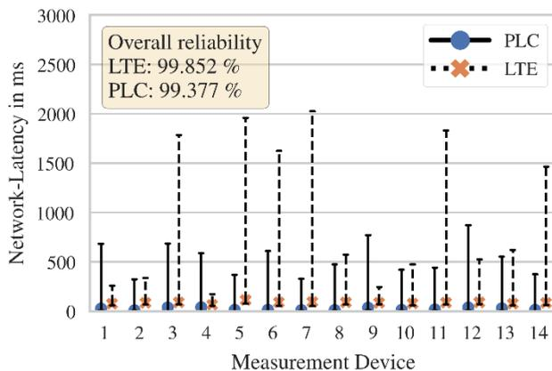
Fig. 3: Minimum, maximum and average network-latency for ping tests executed every second over 24 hours
