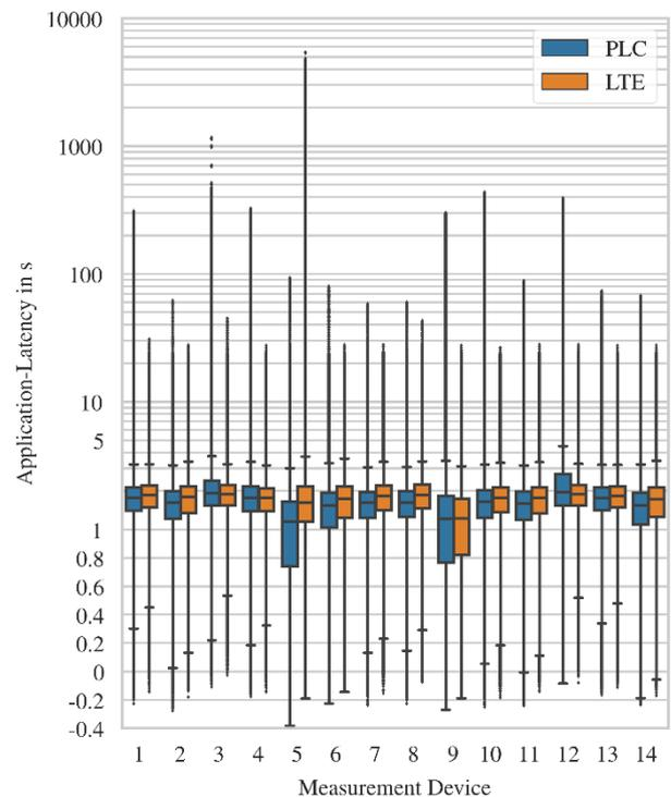
Fig. 4: Comparison of the application-latency for a test period of seven days at an interval of one second
