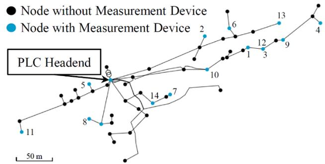
Fig. 2: Placement of measurement devices within the power system of the field-test
