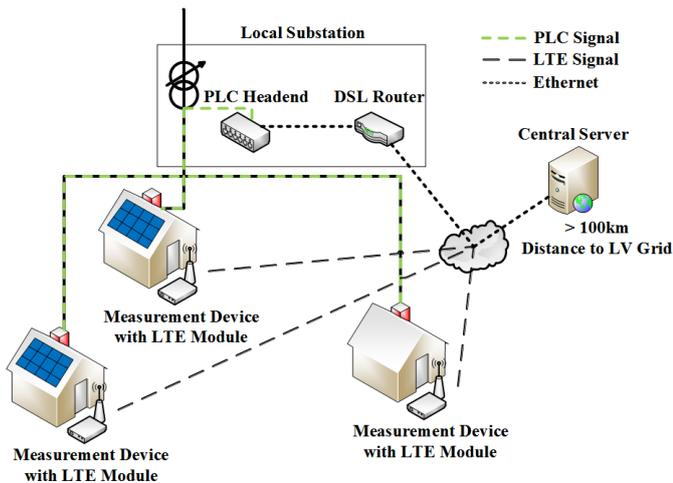
Fig. 1: Communication concept for measurement and control signals using PLC and LTE simultaneously
