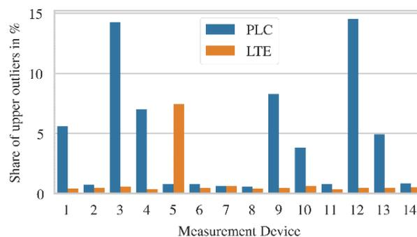
Fig. 5: Comparison of the share of upper outliers in the application-latency distribution per measurement device
