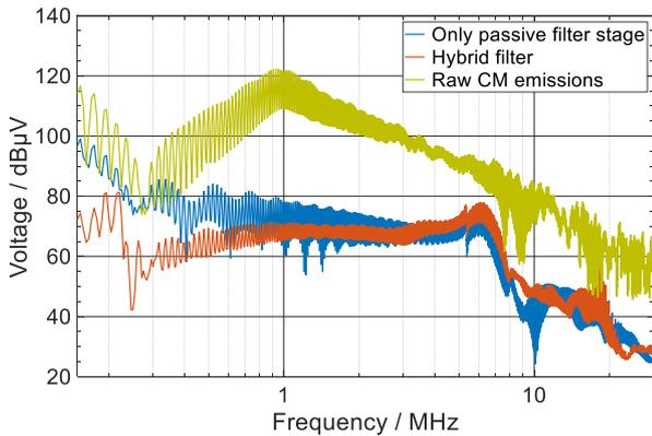
**Fig. 5:** Measurement of conducted CM emissions at LISN
