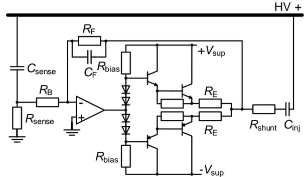
**Fig.2:** Equivalent single phase circuit of the active feedback filter stage
