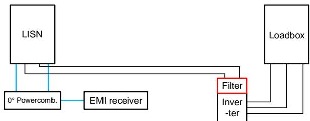
Fig. 4: Test setup according to CISPR25
