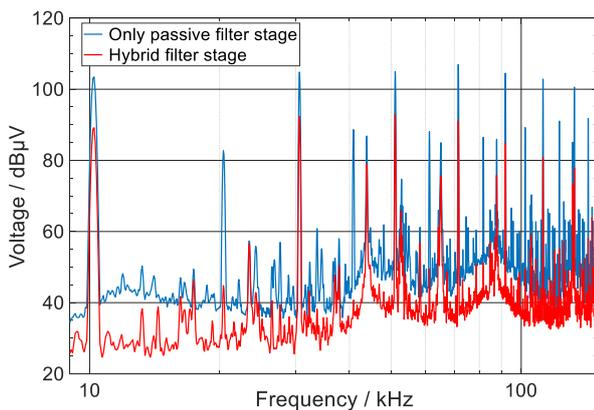
**Fig. 6:** Measurement of conducted CM emissions at LISN for frequencies below 150 kHz
