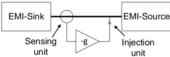
**Fig. 1:** Block diagram of an active feedback EMI filter
