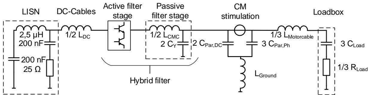
Fig. 3: Single phase CM equivalent circuit of the test setup with active and passive filter stage
