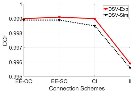
**Figure 9.** Sensitivity comparison of different connection schemes to detect DSV (between disk 2&3)
