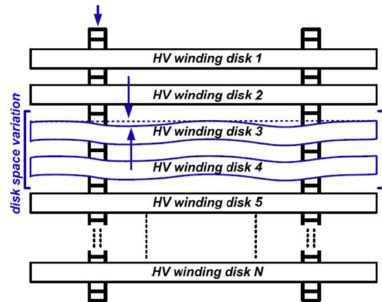
**Figure 4.** Disk space variation between disk 2 and 3 of transformer HV windings [19].
