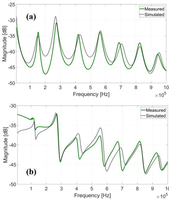
**Figure 3.** Comparison of measurement and simulation for different connection schemes for healthy case of windings
