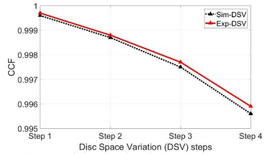
**Figure 8.** CCF of simulated and measured FRA traces (II) for different fault levels of DSV (between disk 2&3)
