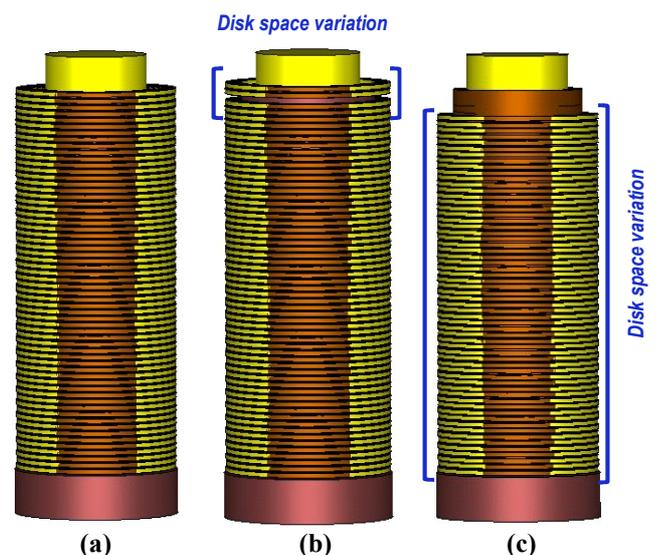
**Figure 5.** Different modes of DSV fault (a) healthy winding (b) DSV between disk 2 and 3 (c) DSV in full winding
