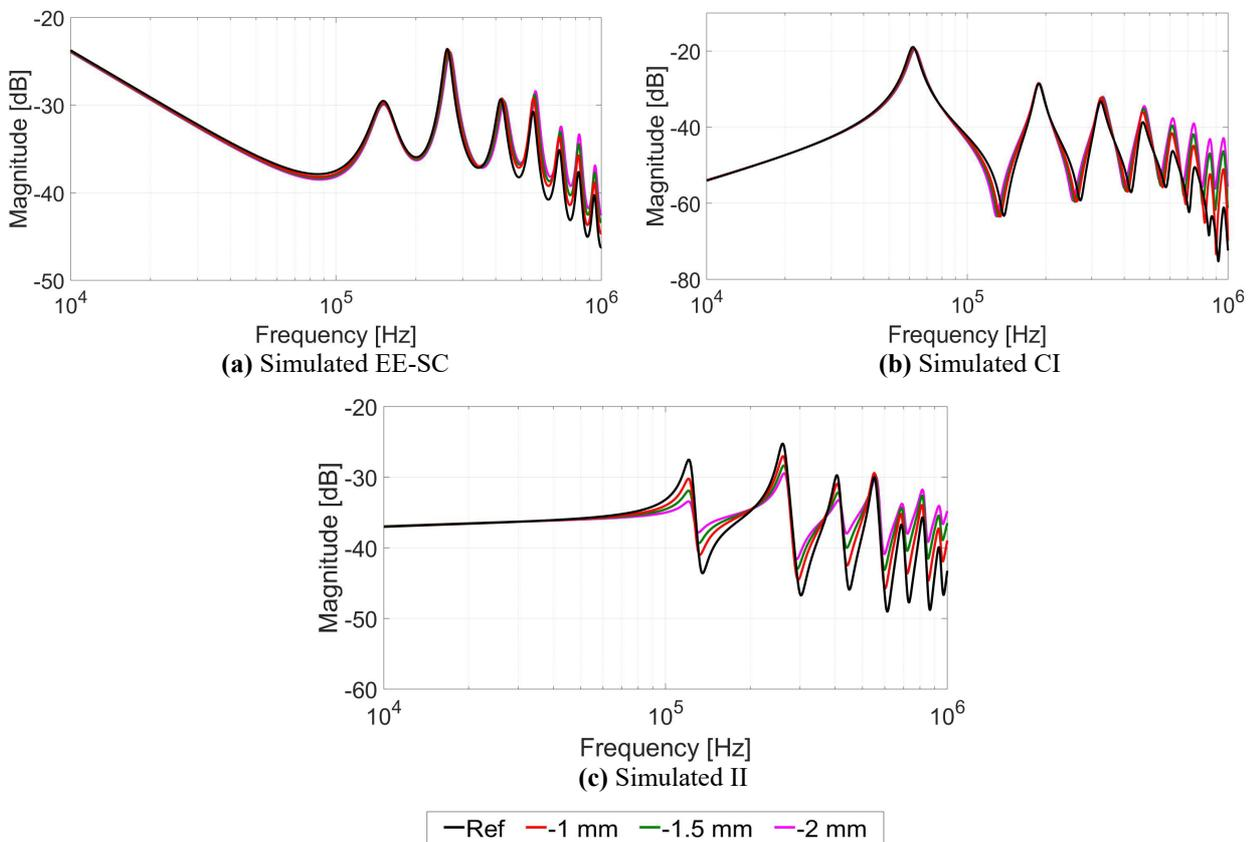
**Figure 7.** Simulated FRA traces for different levels of DSV in full winding
