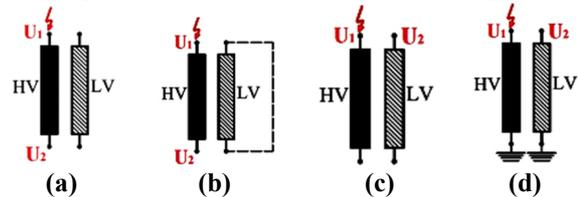
**Figure 2.** Connection schemes for FRA measurement (a) end-to-end open circuit (EE-OC) (b) short circuit (EE-SC) (c) Capacitive inter-winding (CI) (d) Inductive inter-winding (II) [8, 9]
