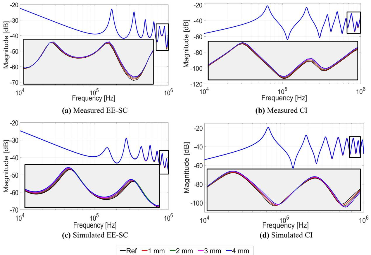
**Figure 6.** Measured and simulated FRA traces for different levels of DSV between disk 2 and 3
