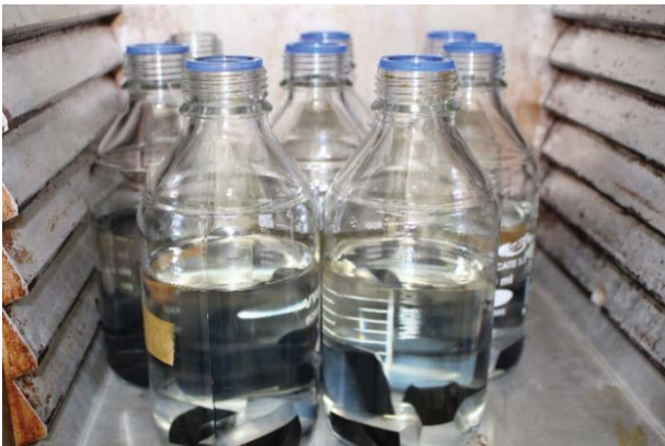
Figure 1 Oil impregnation of solid insulation materials
