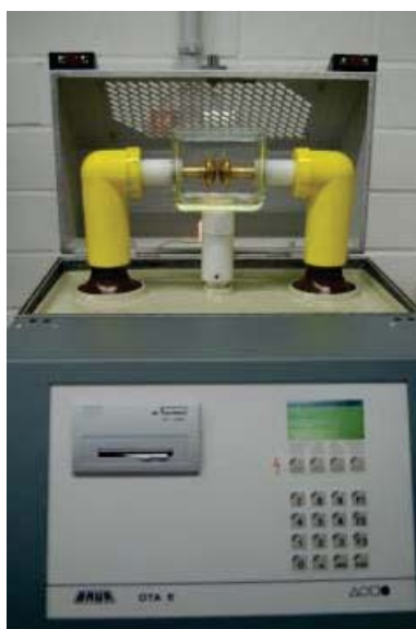
Figure 2 Breakdown Voltage (BDV) Determination equipment
