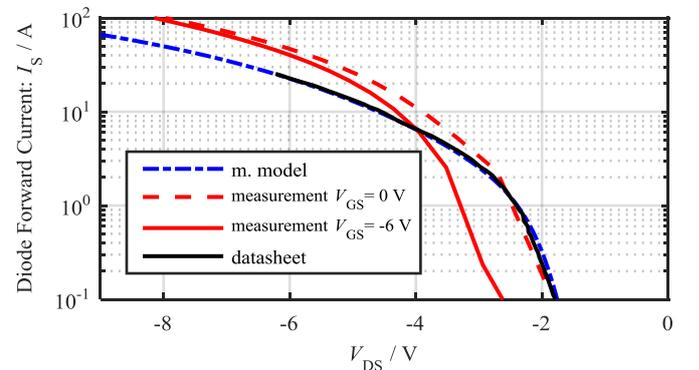
Fig. 5. Comparison of diode output characteristics at different gate voltages.
