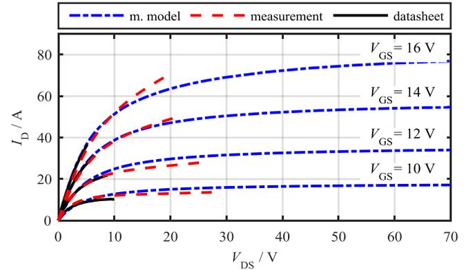
Fig. 4. Comparison of IV curves of the MOSFET in the first quadrant.
