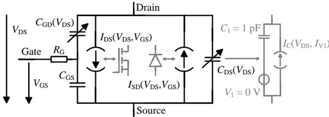
Fig. 2. Circuit elements of the behavioral MOSFET model.
