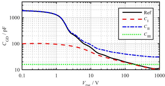
Fig. 15. Comparison of the voltage-dependent space-charge capacitances.
