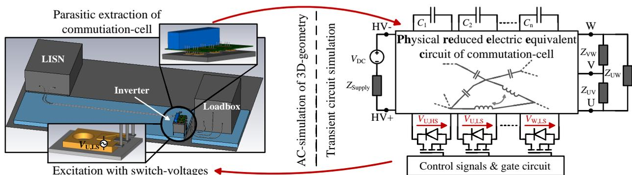
Fig. 1. General simulation approach: Combine the transient circuit simulation of the commutation cell with 3D AC simulation of the complete test setup.
