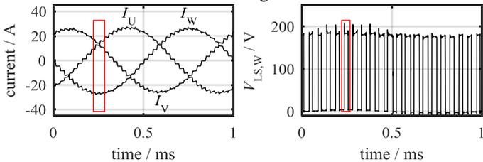
Fig. 8. Time domain simulation result of one load cycle. Left: Load currents of 3-load. Right:  $V_{DS}$  of the low-side MOSFET (halfbridge W).
