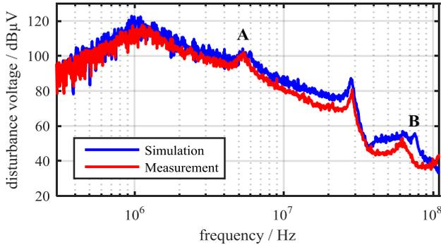
Fig. 11. Comparison between simulated and measured disturbance voltage.
