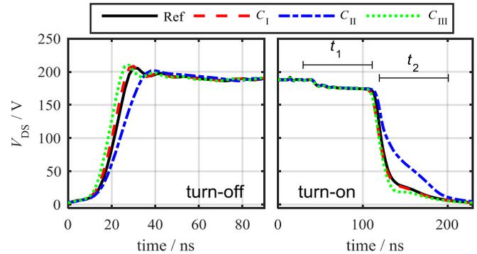
Fig. 16. Time domain simulation results for the capacity variations.
