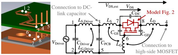
Fig. 6. Computing the necessary parasitic elements from the 3D model.
