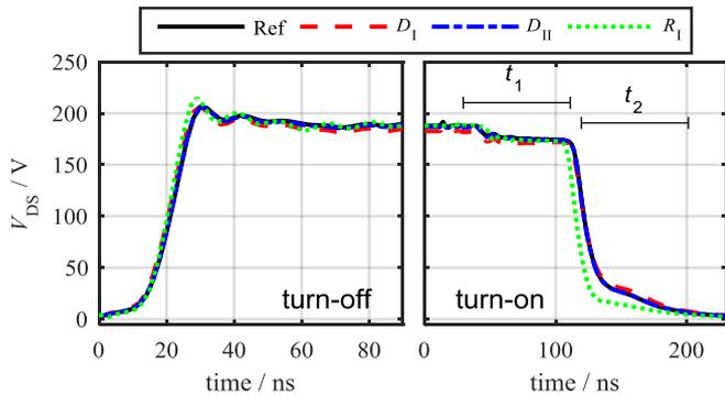
Fig. 18. Time domain simulation for the diode and gate resistance variations.
