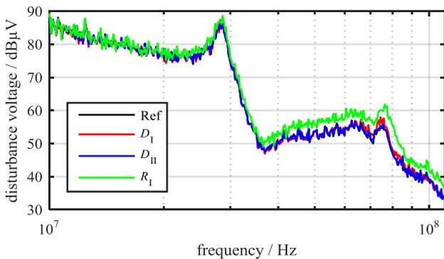
Fig. 19. AC simulation results for the diode and gate resistance variations.
