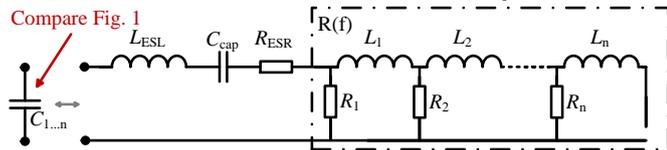
Fig. 7. Equivalent circuit used for DC-link capacitors.
