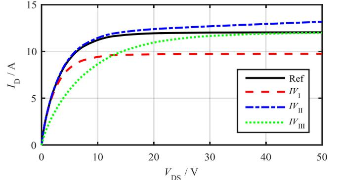
Fig. 12. Variation of IV curves of the MOSFET shown at  $V_{GS} = 10$  V.
