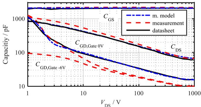
Fig. 3. Comparison of MOSFET capacitances.
