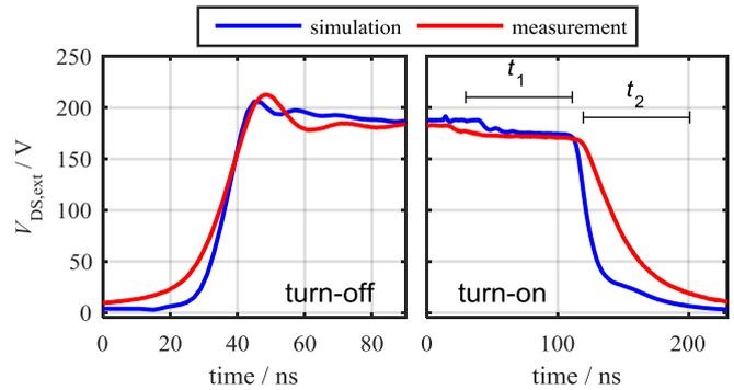
Fig. 9. Comparison of the time domain simulation result with measurements.
