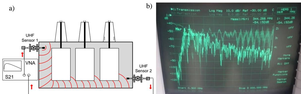
Figure 10: a) Transmission measurement from UHF sensor to UHF sensor through a transformer
