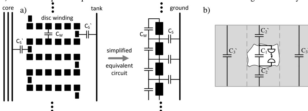
Figure 2: a) Transformer disc winding as low-pass filter for electrical PD signals
