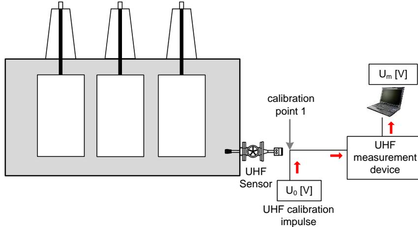
Figure 11: Calibration of measurement device and cables
