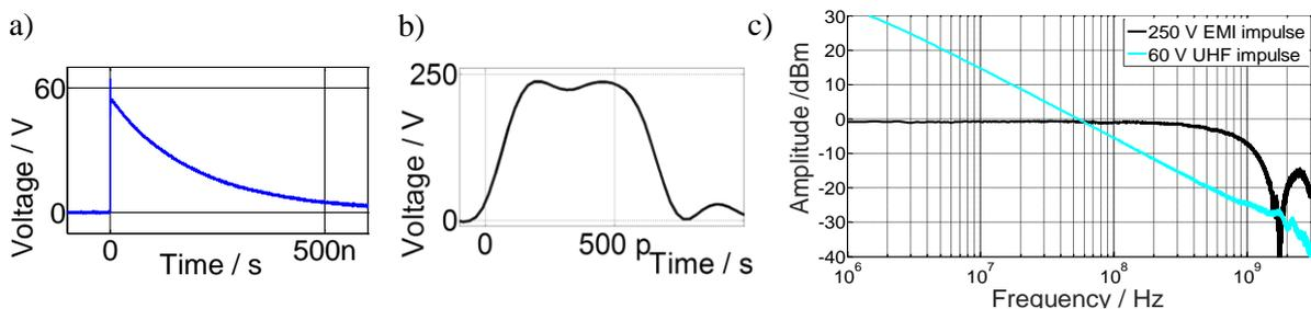
Figure 9: a) 60 V impulse of UHF impulse generator
