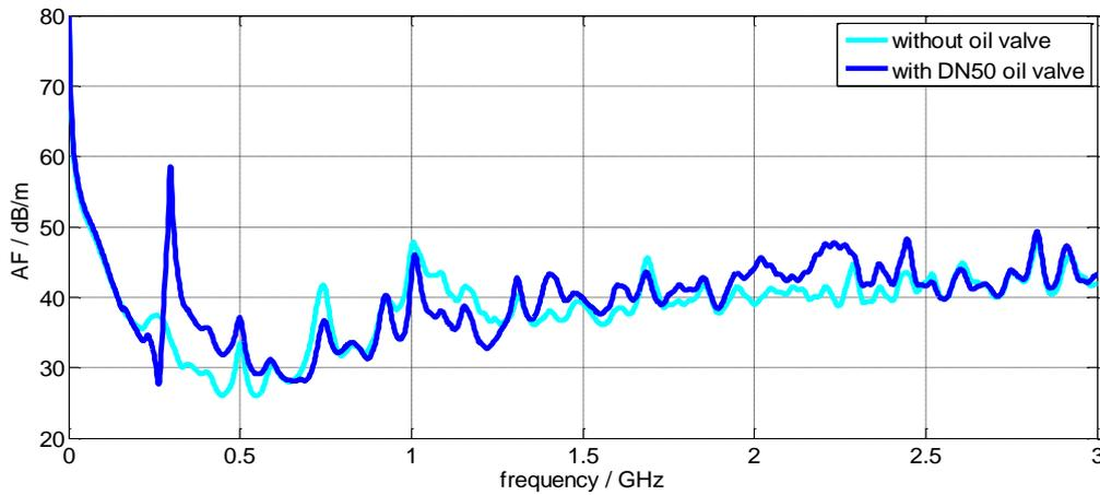
Figure 7: Antenna factor (AF) of UHF sensor measured in GTEM cell
