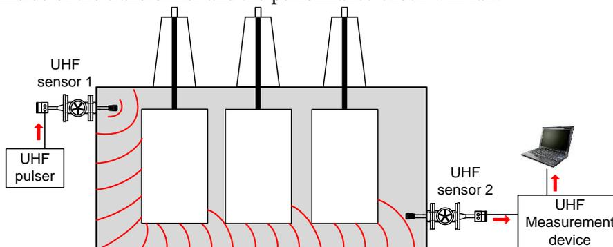
Figure 8: Performance check of UHF PD measurement
