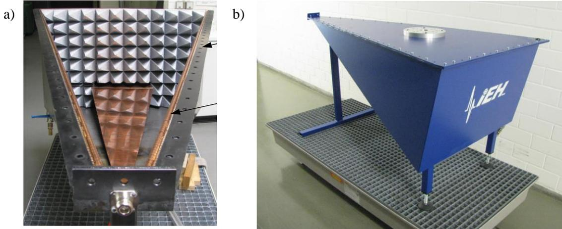
Figure 5: a) GTEM cell internal view with absorbers and septum before oil filling
