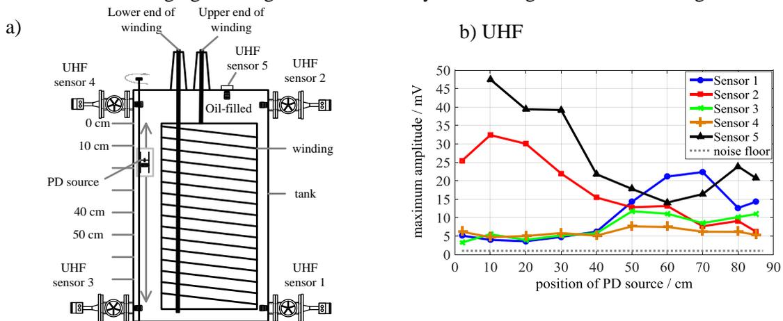
Figure 3: a) Test setup for both electrical PD measurement (IEC60270) and UHF measurement b) maximum measured UHF levels of UHF sensors 1-5 [11]
