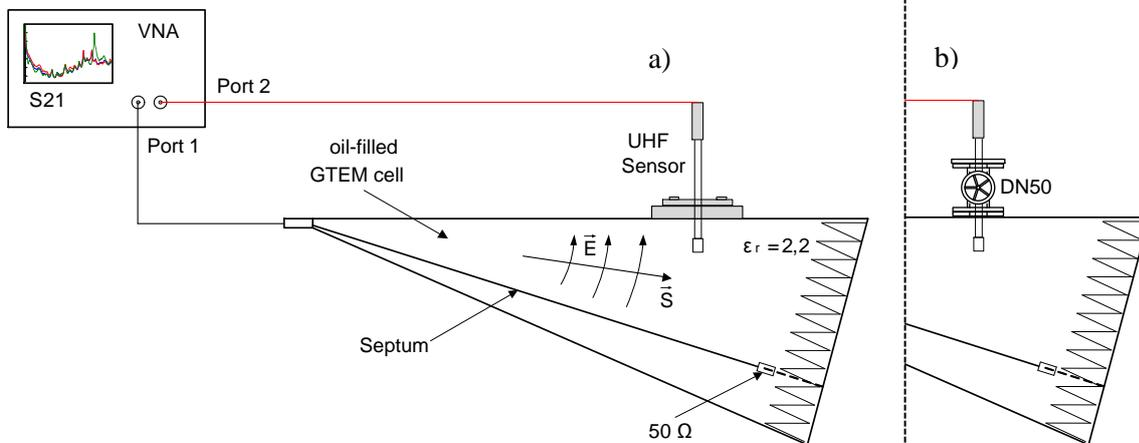
Figure 6: Transmission measurement ( $S_{21}$ ) for AF determination
