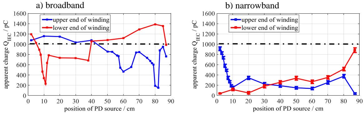
Figure 4: Apparent charge of electrical PD measurement at upper and lower end of winding; dotted line: Actual charge of the source [11]
