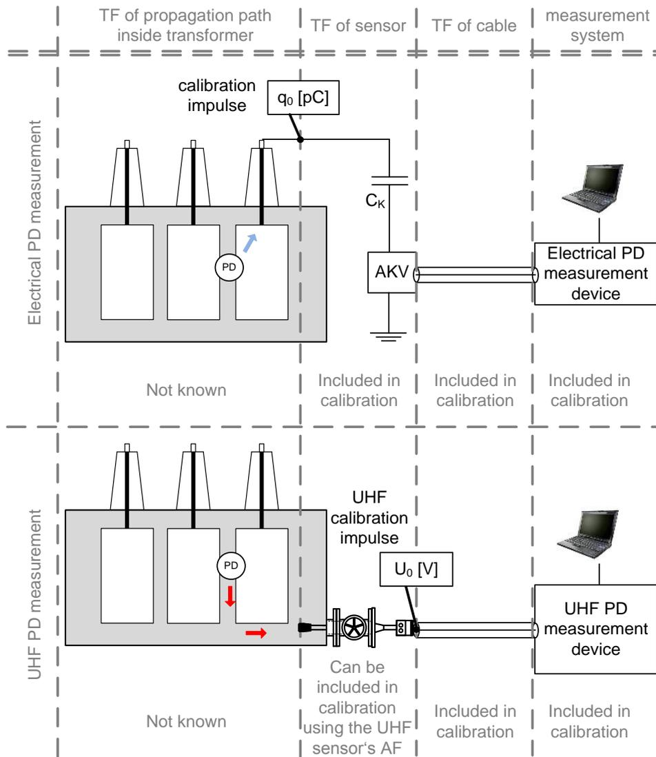
Figure 13: Comparable calibration achievements of electrical and UHF measurements
