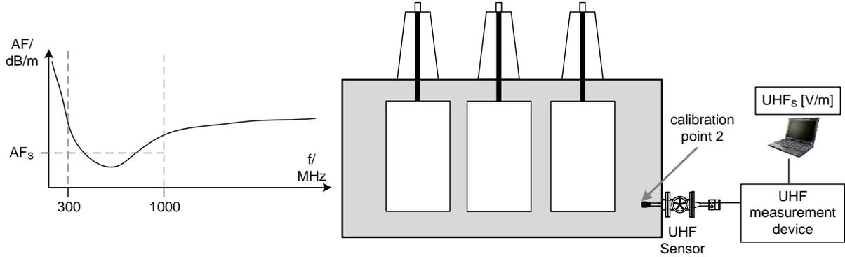
Figure 12: Calibration of the UHF Sensor
