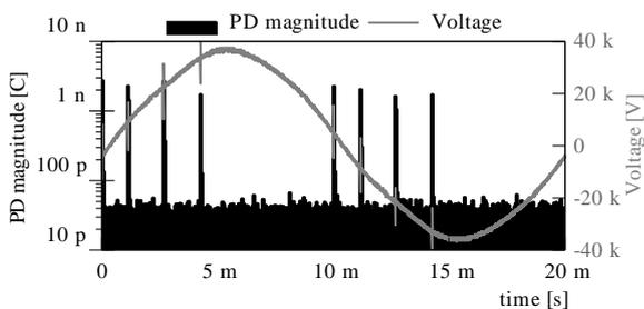
**Figure 8** Phase resolved PD pattern at 20 kV and AC 50 Hz voltage. The magnitude of PD is about 2 nC. The PD source is connected to the cable system located at near end.
