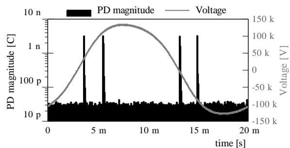
**Figure 9** PD measurement with the artificial PD source and 50 Hz voltage excitation. The phase relation of the PD is at the zero crossing of the voltage.
