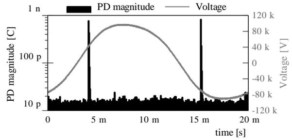
**Figure 11** PD pattern by 50 Hz alternating current excitation with a voltage of 68 kV. The artificial PD source is placed at Joint 1 and the measurable magnitude is 800 pC.
