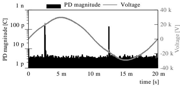
**Figure 6** Phase resolved PD pattern at 16 kV and AC 50 Hz voltage. There is one ignition of the artificial PD source with a magnitude of about 150 pC. The PD source is located at Joint 1 without cable system.
