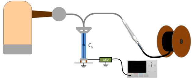
**Figure 2** Test setup for the 50 Hz AC measurement. The high voltage transformer is connected to the cable system and in parallel the coupling capacitor with the PD detection unit is connected. The coupling capacitor is connected in the base point to a digitizer card by a coupling device.
