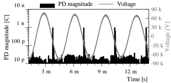
**Figure 12** PD pattern with damped AC voltage shape and a charging voltage of 82 kV. The artificial PD source is placed at Joint 1 and has a magnitude of 950 pC.
