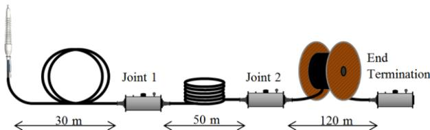
**Figure 1** Test setup with air termination on the left side, 3 sections of high voltage cable, two joints and one SF6 filled termination.
