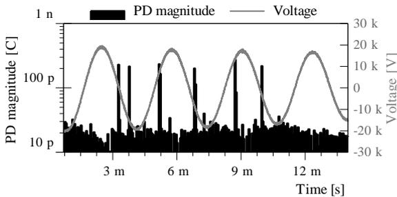
**Figure 10** DAC measurement plot with PD detection. The PRPD pattern shows partial discharges from the artificial PD source near to the voltage zero crossing.
