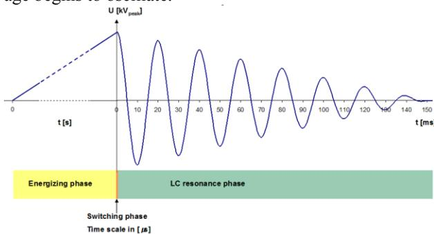
**Figure 4** Typical DAC voltage shape. The RMS-value of the voltage is determined by  $V_{\text{DAC}}/\sqrt{2}$  of the 1st cycle.
