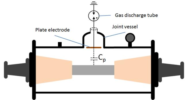
**Figure 5** Schematic view on the artificial PD source placed in a joint. The cable is connected through a cable socket to the inner conductor of the joint.
