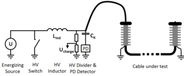
**Figure 3** DAC test circuit connected to the cable under test.
