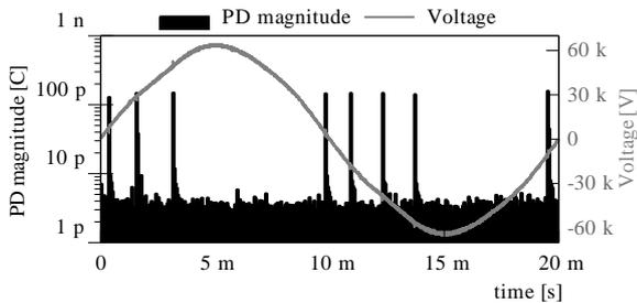
**Figure 7** Phase resolved PD pattern at 45 kV and AC 50 Hz voltage. There are four ignitions of the artificial PD source with a magnitude of about 150 pC. The PD source is located at Joint 1 without cable system.
