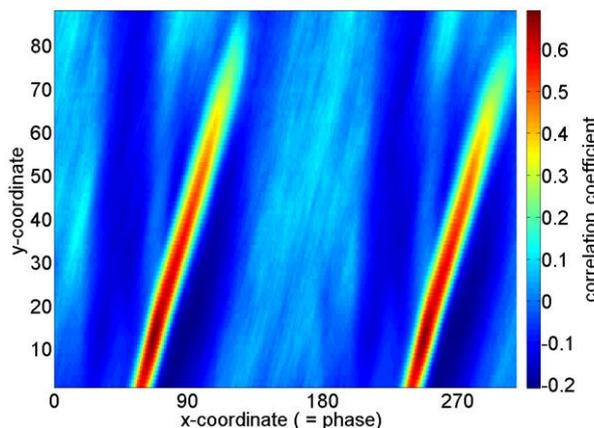
**Figure 4:** Visualization of the correlation matrix of normalized cross-correlation vs. phase in degree. Colour indicates the similarity between template and picture [9].
