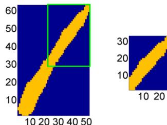
**Figure 3:** Examples of two binary templates of different size. Left: larger template defining the entire shape of the considered pattern. Right: smaller template generated as cut-out of the large template [9].
