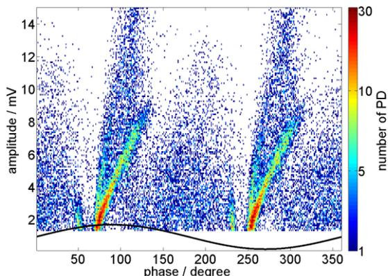
**Figure 2:** PRPD pattern from UHF measurement (one minute record time), called pattern 1
