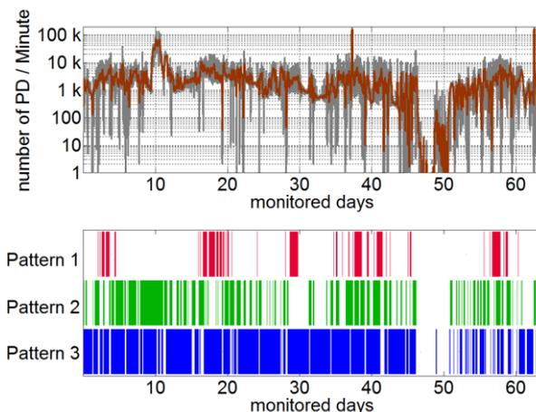
**Figure 9:** PD activity and occurrence of patterns. Upper plot: number of PD per minute (grey) and moving average (brown) Lower plot: results of recognition algorithm of determined patterns 1 - 3 over the monitored time.
