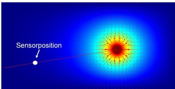
**Figure 14:** Simulation of the electrical field strength in the test tank setup at applied voltage  $V_{RMS} = 70$  kV
