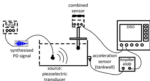
**Figure 5:** Laboratory test setup for reproducible acoustic PD measurements
