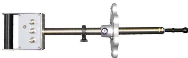
**Figure 1:** Combined sensor for UHF PD, acoustic PD and vibration measurement. Right: sensor head, middle: oil valve adaptor, left: three N-connectors for separated signal outputs
