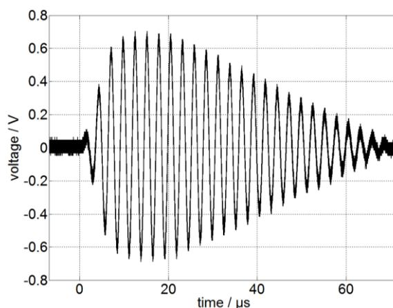
**Figure 6:** PD signal generated by direct digital synthesis (DDS) with variable parameters: frequency, rise time and fall time (here: 180 kHz, 4 periods rise and 10 periods fall time)
