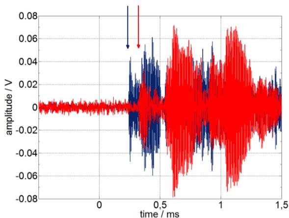
**Figure 7:** Signal of in-oil (blue) and outside tank wall measurement (red). PD signal frequency 150 kHz
