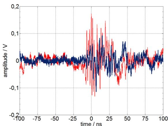
**Figure 12:** UHF measurement of needle-sphere electrode. Red: UHF antenna, Blue: UHF output of diplexer from combined sensor
