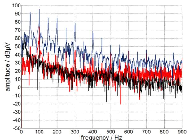
**Figure 13:** Frequency spectrum of vibration measurement at 100 Hz excitation. Blue: in-oil measurement of combined sensor
