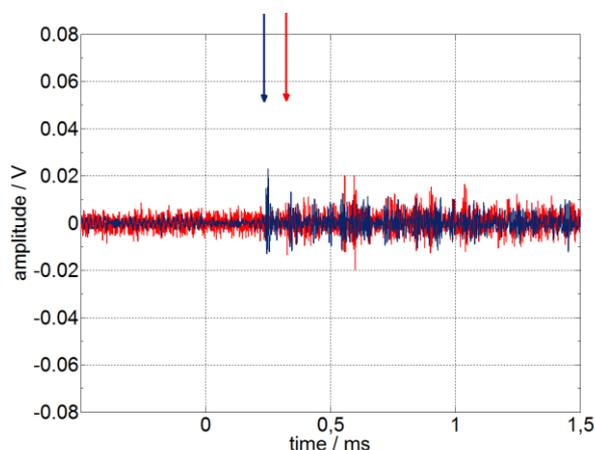
**Figure 8:** Signal of in-oil (blue) and outside tank wall measurement (red) at 40 dB amplification. PD signal frequency 180 kHz
