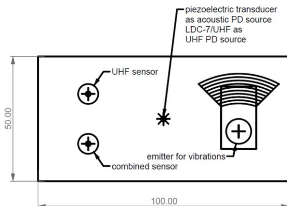
**Figure 4:** Laboratory test setup for combined PD and vibrations measurements
