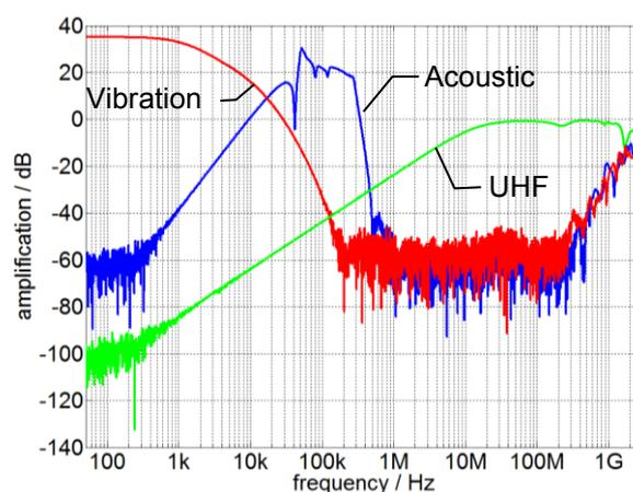
**Figure 3:** Transfer function of diplexer, red: low pass filter for vibration measurement blue: band-pass filter for acoustic PD (both active), green: high pass filter for UHF PD (passive)
