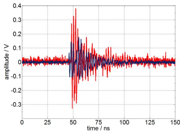
**Figure 10:** UHF measurement of LDC-7 pulser. Red: UHF antenna, Blue: UHF diplexer output
