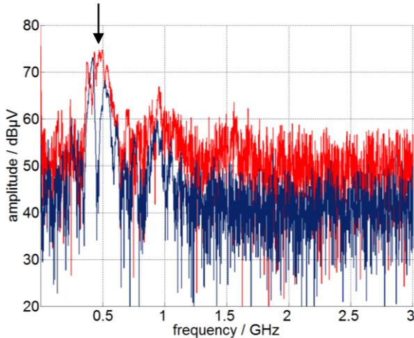
**Figure 11:** Frequency spectrum of time domain measurement from Figure 10. Red: UHF antenna, blue: UHF output of diplexer from combined sensor
