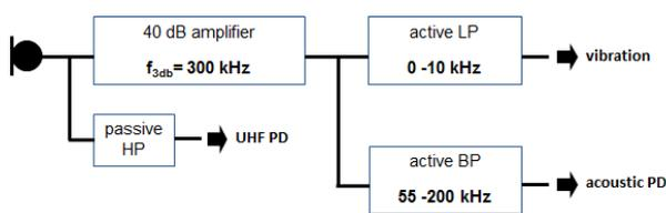
**Figure 2:** Block diagram of diplexer to separate signals from UHF PD, acoustic PD and sinusoidal vibration signals to separate outputs. On the left: sensor receiving all signals simultaneously
