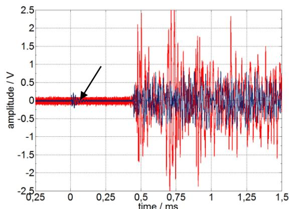
**Figure 9:** Acoustic measurement of needle-sphere PD source, triggered on UHF antenna. Low frequency coupling of electromagnetic components in combined sensor
