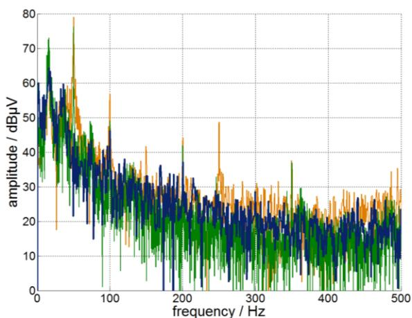
**Figure 15:** Frequency spectrum comparing vibration measurement and influence of the electric field. blue: noise measurement of combined sensor green: coupling at  $E_{RMS} \sim 9$  kV/m, orange: coupling at  $E_{RMS} \sim 22$  kV/m
