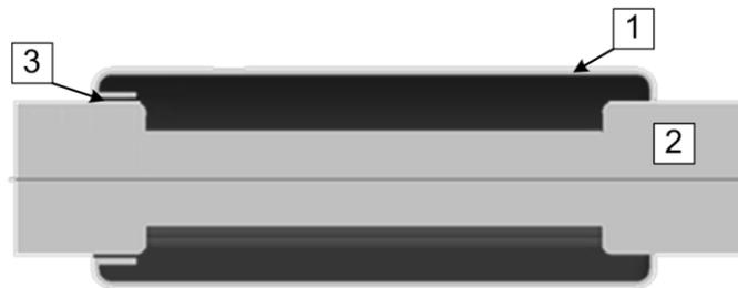
Figure 12: Schematic drawing of a resonator: An aluminium tube (1) is arranged around the inner conductor of the GIS (2). A long and thin gap (3) between resonator and conductor is formed on one side of the tube.
