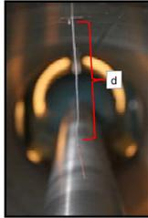
Figure 4. The hanging particle to represent the height of the particle jump.
