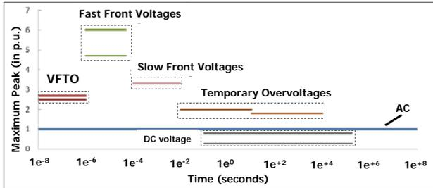
Figure 1. Different Voltage Stresses during the Operation of GIS [2]
