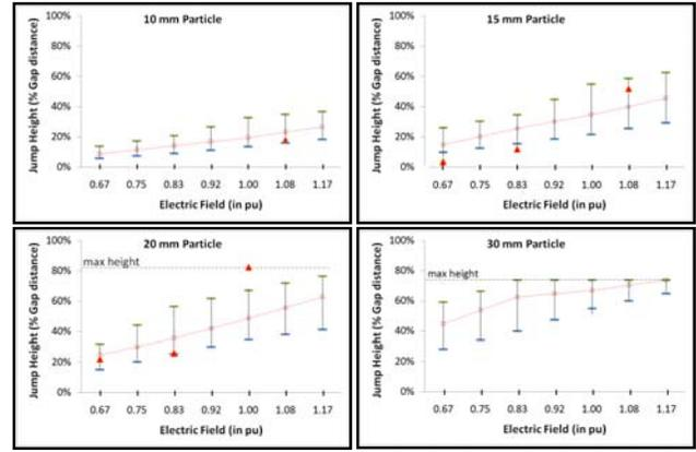
Figure 5. The maximum jump of different particles under AC voltage 1 p.u.
