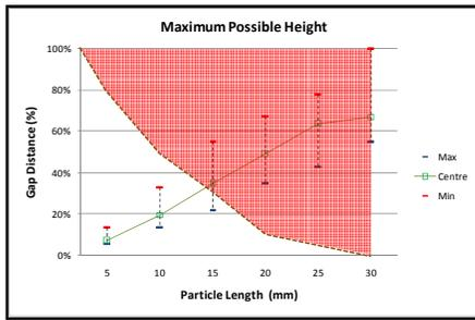
Figure 7. The breakdown area based on the experiments with LI and the simulation works under AC voltage.
