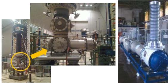
Figure 2. GIS Test Setups Used in the Experiments, in TU Delft (left) and in TU Stuttgart (right)
