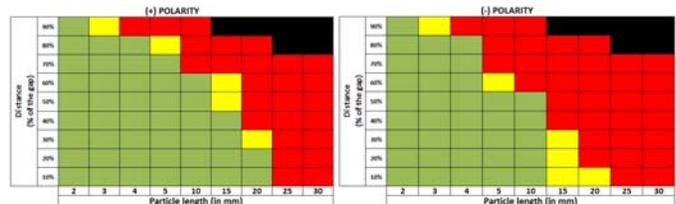
Figure 6. The breakdown matrices under positive (left) and negative (right) LI
