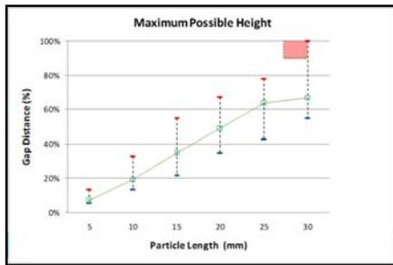
Figure 8. The breakdown area based on the experiments with VFTO and the simulation works under AC voltage
