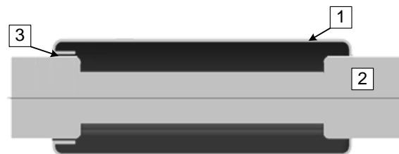
Figure 6: The resonator (1) around the inner conductor of the GIS (2) with a long gap between resonator and conductor (3)
