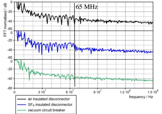
Figure 13. FFTs of the busbar voltage curves.
