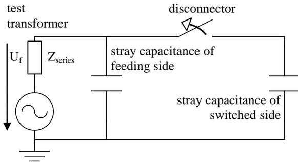
Figure 2. Equivalent circuit diagram for disconnector arcing.
