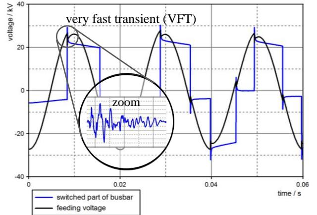
Figure 4. Voltage measurement at busbars.
