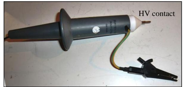
Figure 6. High voltage probe, type LeCroy PPE20KV. The bandwidth of the high voltage probe is 100 MHz (-3 dB point). The attenuation factor is 1000.
