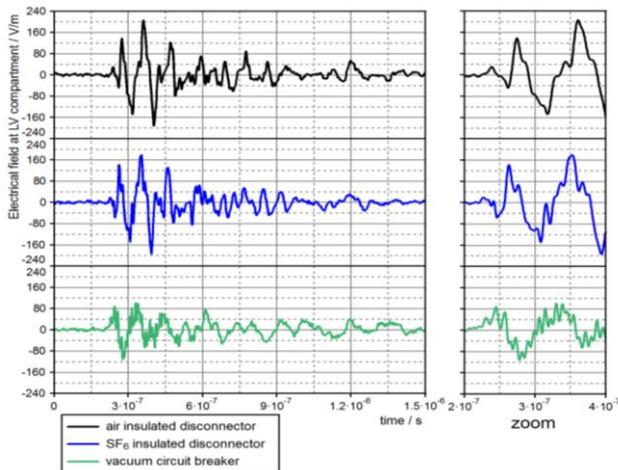
Figure 9. Electrical field measurement.
