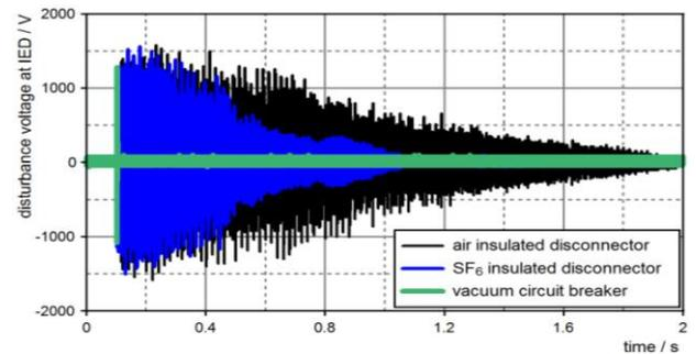
Figure 7. CM disturbance voltage at the IED's CT ports.
