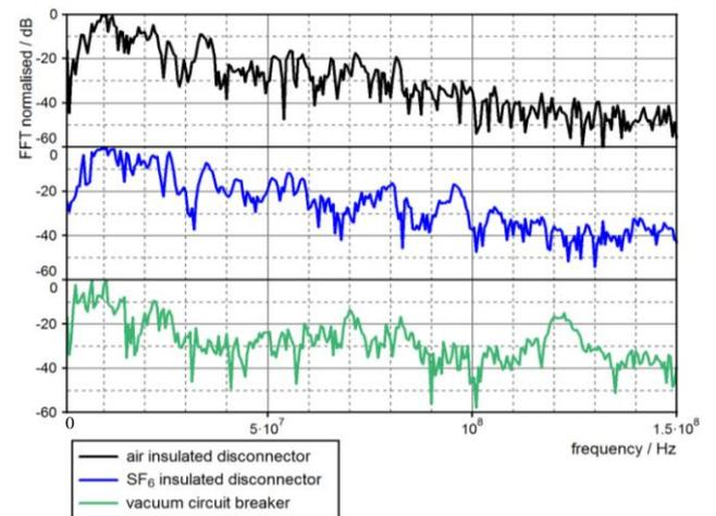
Figure 10. Normalized FFT of electrical field measurement.
