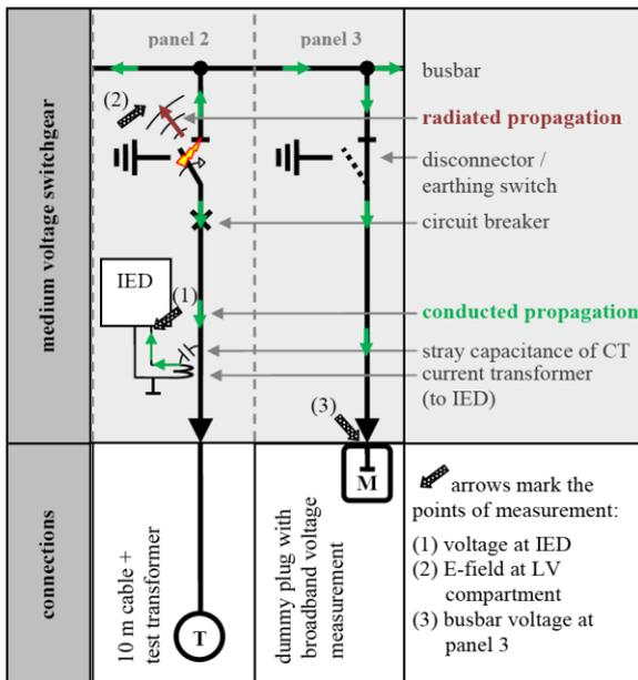
Figure 5. Test setup and measurement points.
