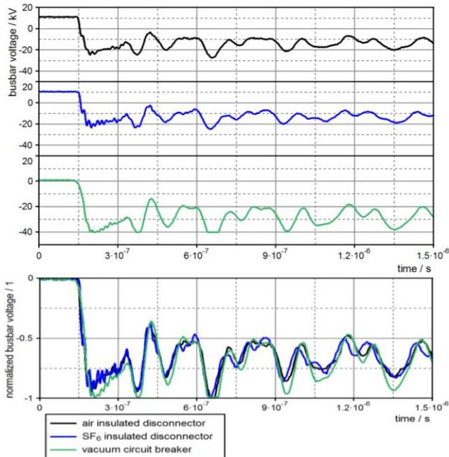
Figure 12. Voltage at the switched part of busbar.
