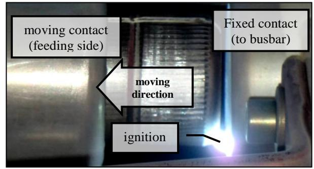
Figure 3. Ignition at the disconnector under test.
