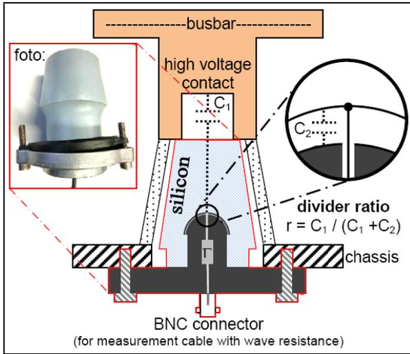
Figure 11. Capacitive voltage divider in a dummy plug. The bandwidth of the voltage sensor is 350 MHz, verified by the measurement of a 4 kV square voltage signal with a rise time of  $t_{rise} \approx 1$  ns.
