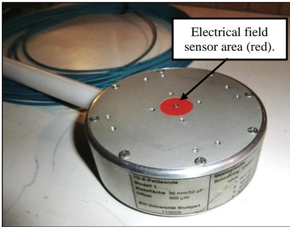
Figure 8. 1-D Electrical field probe. The bandwidth of the electric field probe is 400 MHz (-3 dB point). It was developed and assembled (2006) at the University of Stuttgart, Institute of Power Transmission and High Voltage Technology (IEH).
