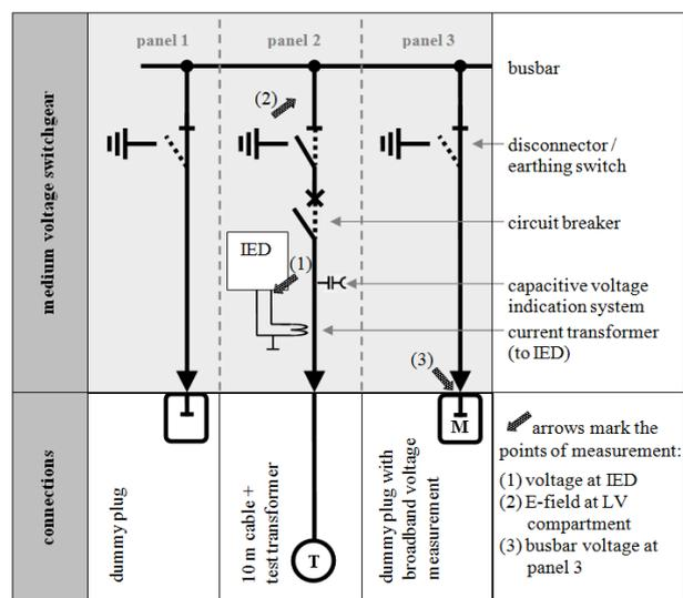
Figure 1. Switchgear test setup.
