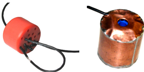
Figure 7 View of sensor, the core of the high-voltage line is fitted through the centre hole
