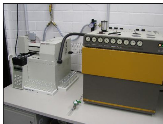
Figure 2: Gas chromatograph with automatic sampler
