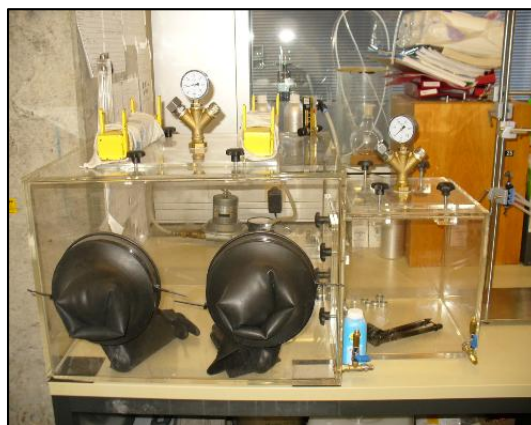
Figure 1: Glove box with argon atmosphere
