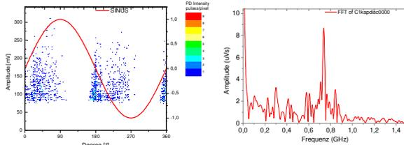
**Figure 10.** Internal PD defect (PRPD and FFT patterns)
