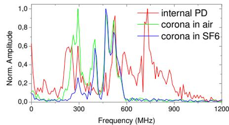
Figure 5. Differentiation between internal and external PDs based on FFT transforms
