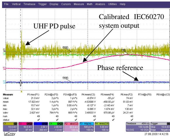
Figure 6. Oscilloscope screenshot
