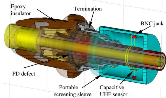
**Figure 1.** Object and principle of the UHF PD diagnostics
