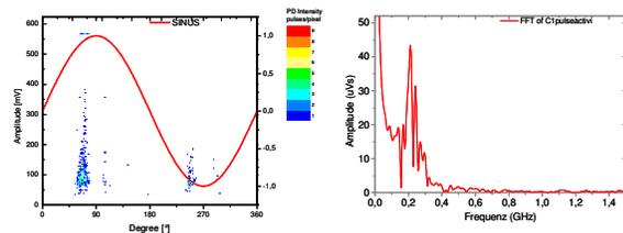
**Figure 9.** On-site test: corona (PRPD and FFT patterns)
