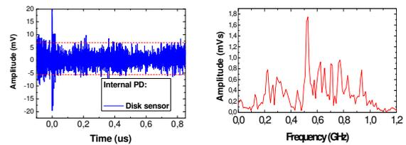
Figure 4. UHF PD pulse of 5 pC (acc. IEC 60270) from the artificial defect in the termination in time and frequency domains
