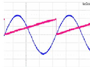
Figure 8. 50 Hz sine form of the applied voltage coupled on-site by the electrode, embedded into epoxy insulator, and a ramped trigger box output signal
