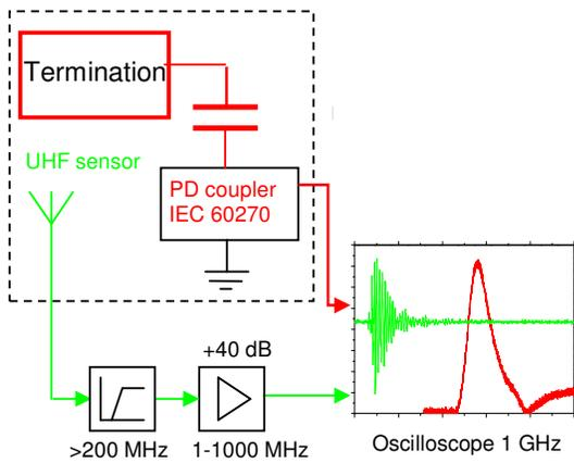
Figure 3. Structural diagram of the comparative measurement between an UHF and IEC60270 PD detecting methods
