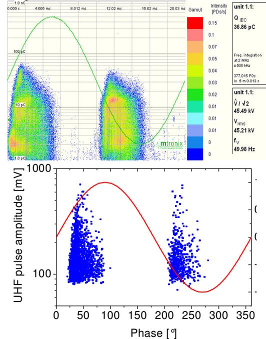
Figure 7: PRPD images of an internal PD (<80 pC at 45 kV) recorded synchronously acc. IEC60270 (left) and using the UHF signal from the oscilloscope (right)
