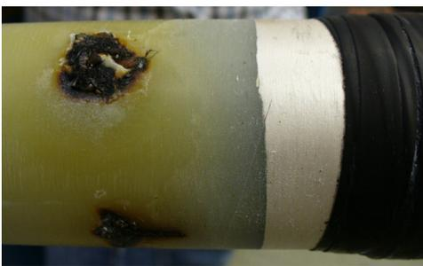
**Figure. 11:** A faulty 72 kV cable termination qualified onsite and dismantled in the lab
