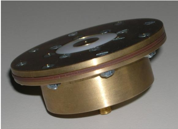
Figure 3. Pommerenke target with integrated PCB. The PCB between the brass material is mounted with the CUT (not visible). The centre electrode surrounded by the white material on the top plane is contacted with the ESD Simulator Gun Tip during ESD Stresses.
