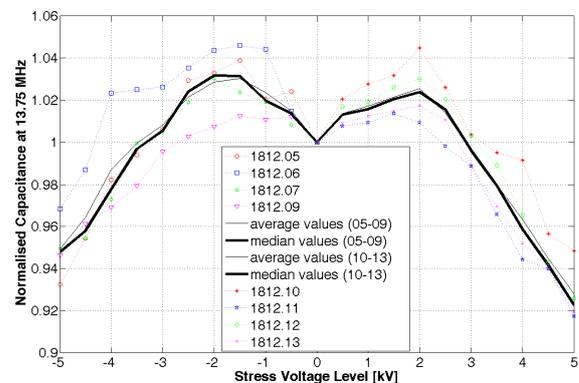
Figure 7. Normalised capacitance value at 13.75 MHz vs. stress voltage level (10 shots per level) for sample type 1812. Four samples were used for each polarity, all measurements are normalised on the respective initial zero voltage values of the sample.
