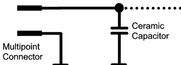
Figure 1. Simplified input circuit diagram of an arbitrary electronic control unit providing a decoupling capacitor directly after the multipoint connector interface.
