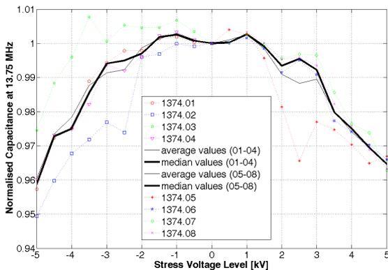
Figure 5. Normalised capacitance value at 13.75 MHz vs. stress voltage level (10 shots per level) for sample type 1374. Four samples were used for each polarity, all measurements are normalised on the respective initial zero voltage values of the sample.
