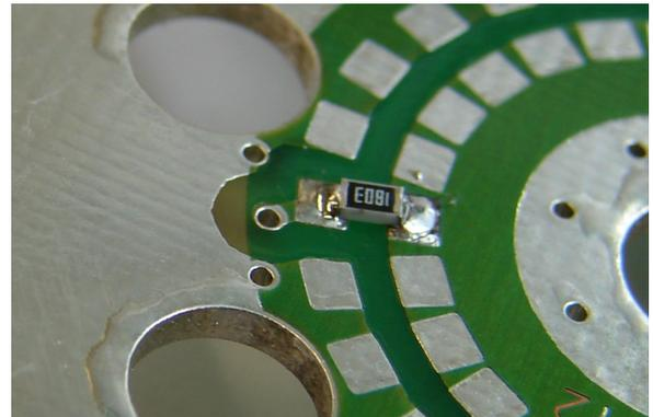
Figure 2. Single surface mounted device soldered to the Pommerenke target PCB. The picture shows the PCB not being integrated into the Pommerenke target.
