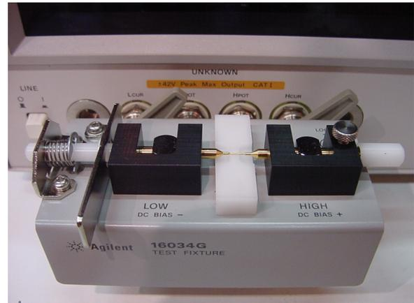
Figure 4. Fixture of the impedance analyser for measuring SMD components. The CUT is inserted between the golden tips in the middle of the fixture during measurement.
