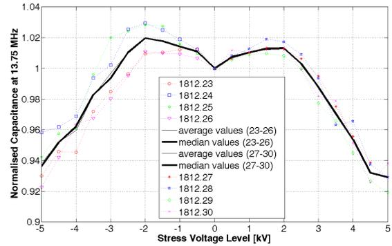
Figure 6. Normalised capacitance value at 13.75 MHz vs. stress voltage level (5 shots per level) for sample type 1812. Four samples were used for each polarity, all measurements are normalised on the respective initial zero voltage values of the sample.
