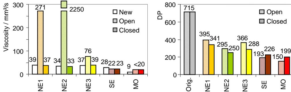
Fig. 2: Ageing experiments with open and closed systems for the natural esters (NE), synthetic ester (SE) and mineral oil (MO); left: kinematic viscosity at 40°C; right: degree of polymerisation of Kraft paper samples aged in the fluids
