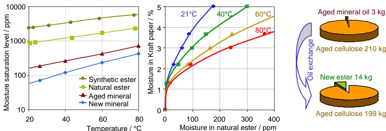
Fig. 1: Left: moisture solubility in synthetic ester, natural esters, aged and new mineral oil, middle: moisture equilibrium chart for natural ester and Kraft insulation paper right: moisture distribution between cellulose and oil for aged mineral oil and after oil exchange for new natural ester at 40°C
