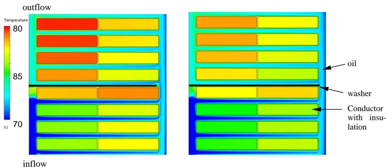
Fig. 6: Temperature distribution in the winding cooled with mineral oil (left) and with natural ester (right) at same flowrate and inlet temperature
