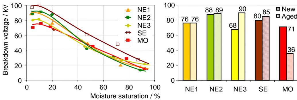
Fig 3: Left: breakdown voltage of esters and mineral oil depending on moisture saturation Right: breakdown voltage before and after ageing at 20 % moisture saturation
