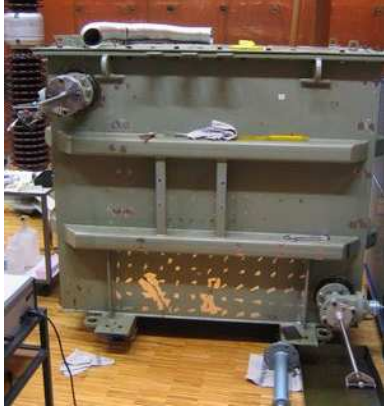
Fig. 9: Test tank with two oil valves and two flange mounted UHF probes
