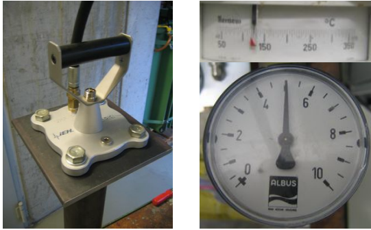
Fig. 2: Picture of leakage test; left) UHF PD probe attached to a test vessel, right) Measured temperature and pressure
