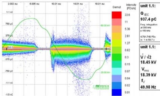
Fig. 4: Phase resolved partial discharge (PRPD) #2.
