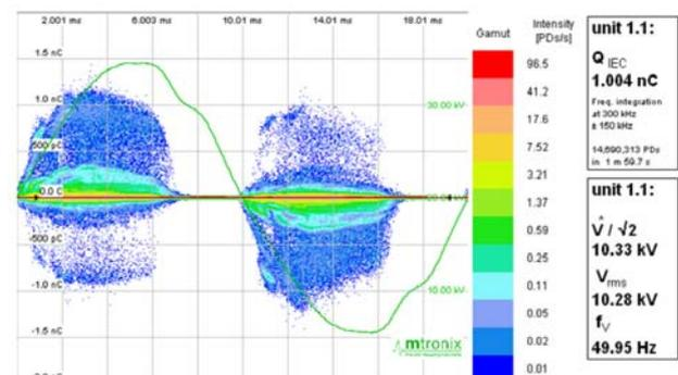
Fig. 2: Phase resolved partial discharge (PRPD) #1.
