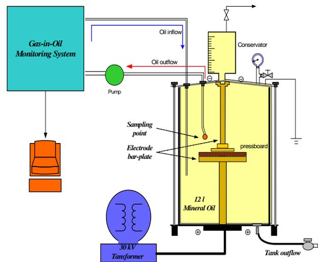
Fig. 1: Test setup for PD-stressing and dissolved gas analysis.
