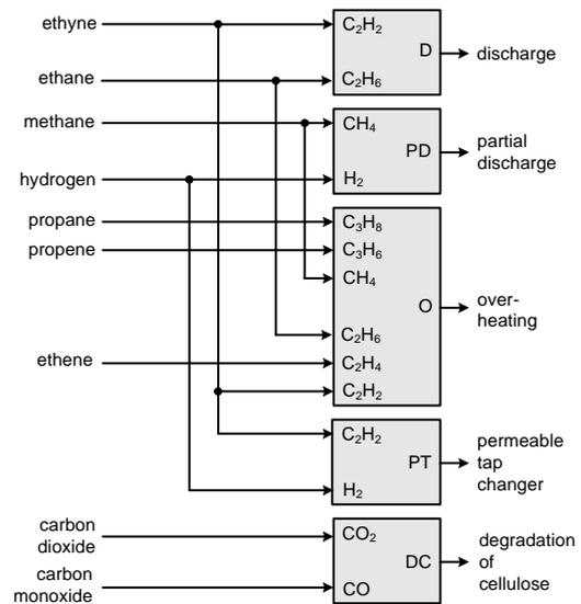
Fig. 7: Considered measurements per type of fault.
