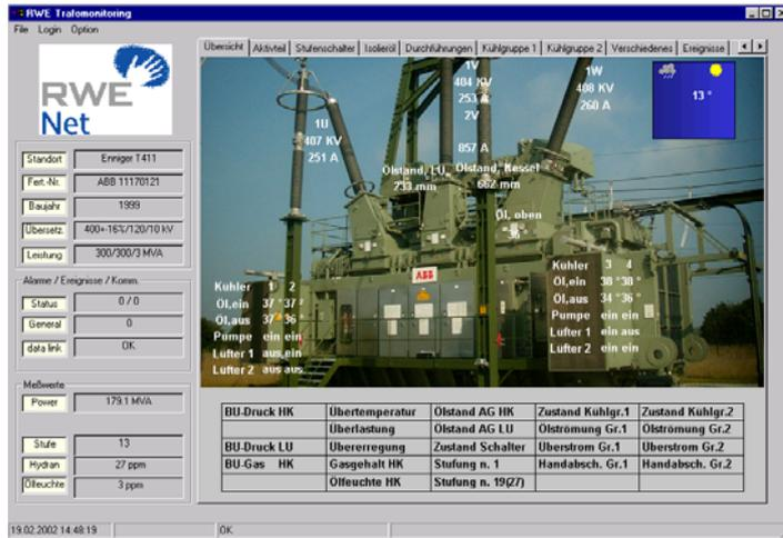
**Fig. 7:** Visualization of the diagnostic quantities and alarm and warning signals of a transformer monitoring system
