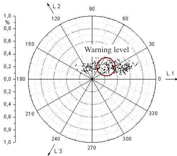
Fig. 8. Polar diagram of the sum vector of a 3-phase bushing monitoring on a 400 kV generator transformer
