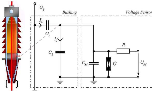
Fig. 3. Sketch of bushing and equivalent circuit diagram of the bushing and the voltage sensor
