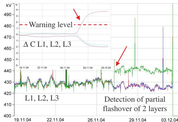
Fig. 6. Detection of partial flashover of 420 kV bushing and avoidance of collateral damage of 350 MVA regulating transformer, 3-phase operating voltages (phase L1, L2, L3) with overvoltages (large fig.), identified by change of capacitance  $\Delta C$  (small fig.)
