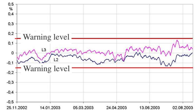
Fig. 7. Changes in the dielectric dissipation factor ( $\Delta \tan \delta$ ) of a 3-phase bushing monitoring system on a 400 kV generator transformer determined on-line
