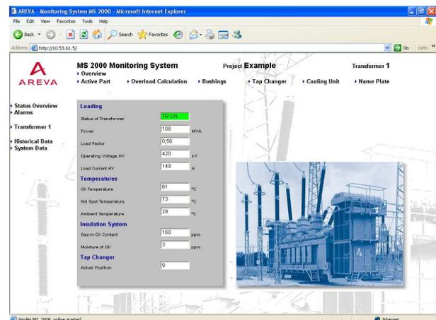
Fig. 1. On-line visualization of transformer condition and its detailed information about trending, diagnostics and prognostics
