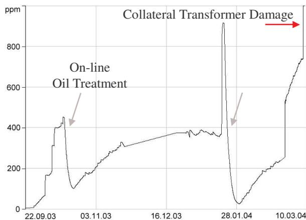
Fig. 10. Gas-in-oil content of a 75 MVA, 33 kV furnace transformer until collateral damage
