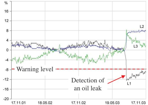
Fig. 9. 3-phase monitoring of the change in the bushing oil pressure on a 400 kV generator transformer with detection of an oil leak on phase L1
