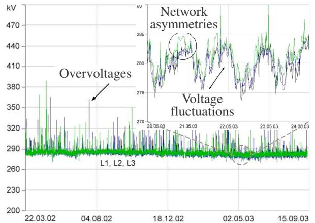
Fig. 5. Continuously monitored 3-phase operating voltages (phases L1, L2, L3) with overvoltages, voltage fluctuations and network asymmetries (period 18 months)
