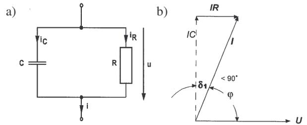
Fig. 2. Equivalent circuit diagram (a) and vector diagram (b) of the dielectric loss factor  $\tan \delta$
