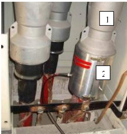
Fig. 4: Test set-up consisting of (1) plug-in connector and (2) metallic barrel sleeve with antennas
