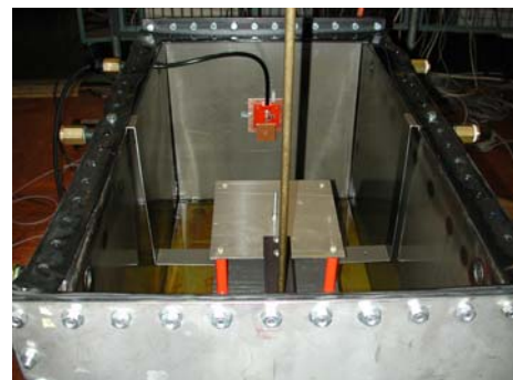
Fig.1: Test tank (1.0x0.5x0.5)m here without cover, prototype monopole (upper middle) and rod-plane PD source (middle of the photo)
