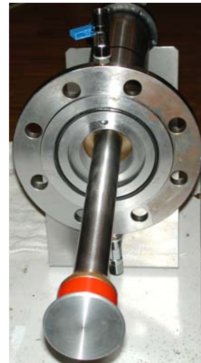
Fig. 10: A disc-shaped UHF-sensor for a standardized valve (DN 80) for online applications
