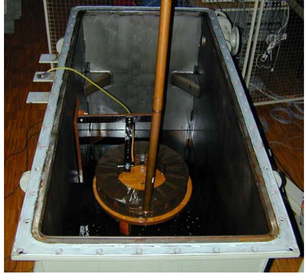
Fig. 5: Transformer tank with high voltage winding, PD stimulated at the inner of the winding at (0.71 / 0.225 / 0.875) m in cartesian coordinates
