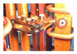
Fig 6: Eroded contacts of the tap selector with a coke layer.
