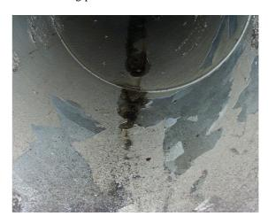
Fig 4: Paint particles from the cooling plant, causing PD
