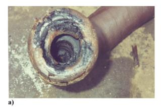
Fig. 8a, b: Connectors with fully burnt out solid insulation
