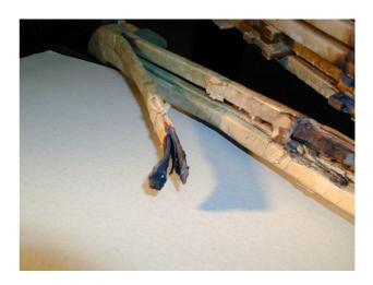
Fig 5: A broken twin conductor as a consequence of a defective solder joint
