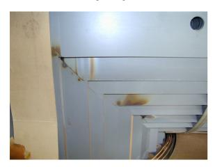
Fig 2: A severe core burn as a consequence of high circulating currents
