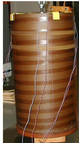
Fig. 1b: Winding equipped with sensors for local temperature measurements.
