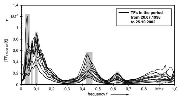
Figure 7: Comparison of several TFs. Recorded between 1998 and 2002 with the same tapping position
