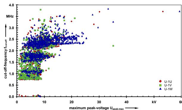
Figure 8: Frequency content of the transient overvoltages on the high voltage side phase
