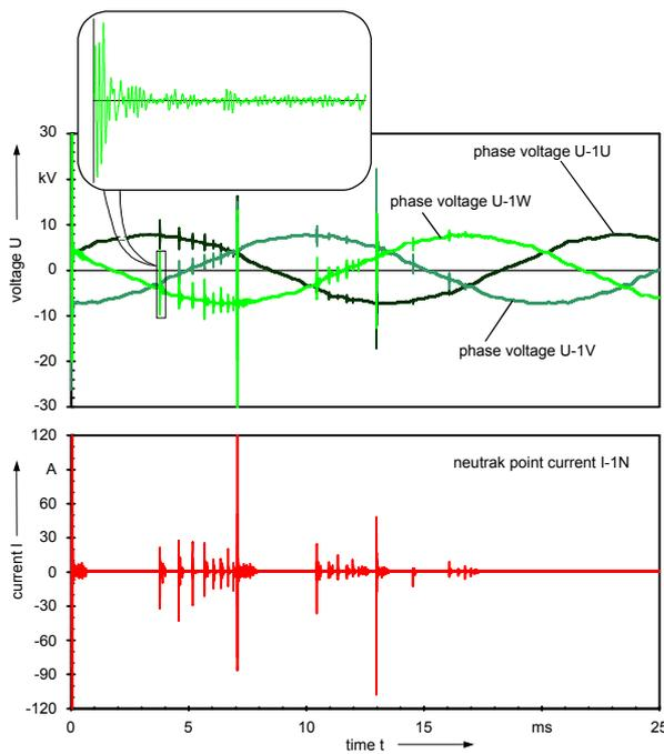
Figure 4: Recorded transient event with zoomed peak. 50 Hz component stronger attenuated as the peaks because of the transfer characteristics of the sensors
