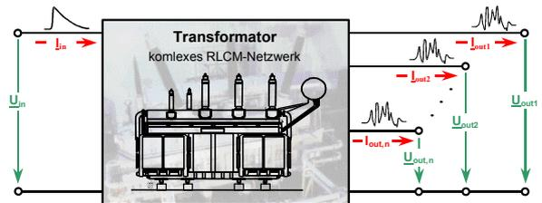
Figure 1: The transformer as a two port
