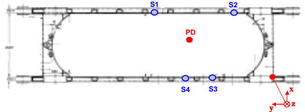
Figure 8: Top view of the housing of a 200 MVA transformer with four acoustic sensors on his outside and the PD location inside
