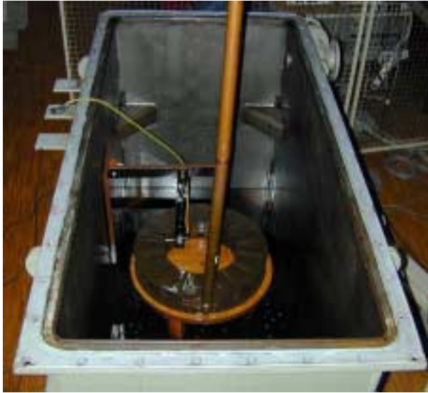
Figure 7: Transformer tank with high voltage winding
