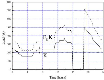
**Figure 2:** Daily diagrams in a short-time emergency loading.
