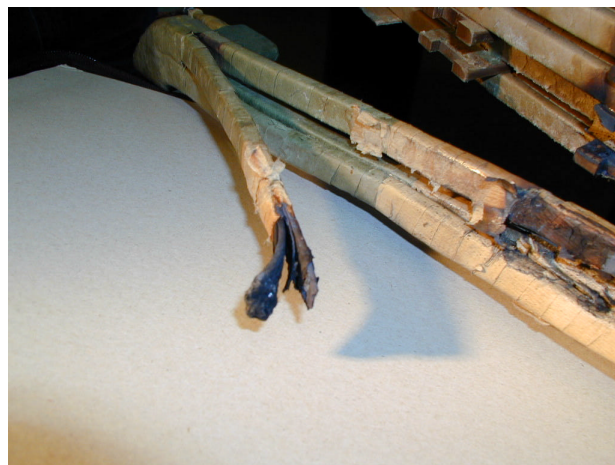
Fig 5: A broken twin conductor as a consequence of a defective solder joint
