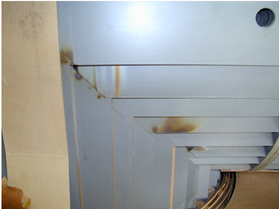
Fig 2: A severe core burn as a consequence of high circulating currents
