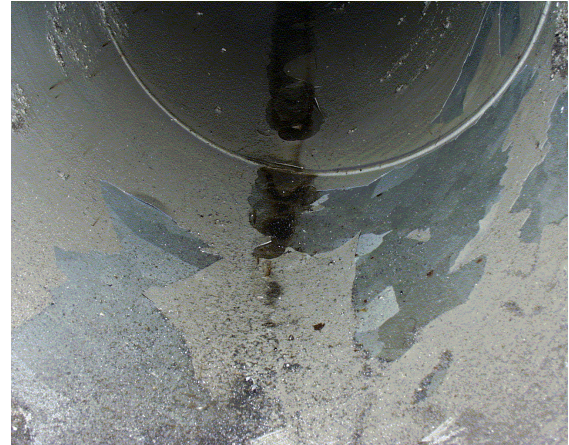
Fig 4: Paint particles from the cooling plant, causing PD
