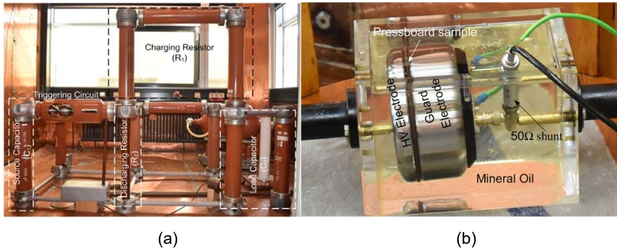
Fig. 1: a) Setup for generating impulse voltage in laboratory. b) Current measurement setup of scaled down insulation model.
