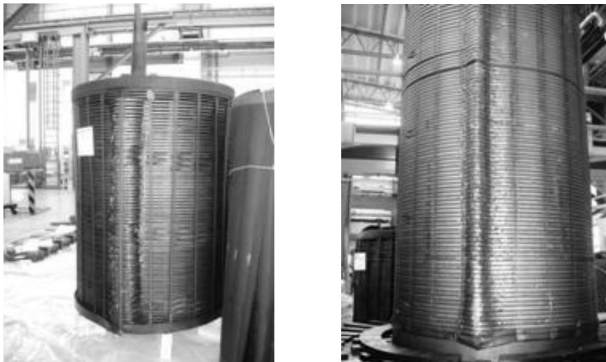
Fig. 1: Kurzschlusschaden (Radiale Deformation) an 220kV/110kV-Wicklungen Short circuit damage (radial deformation) at 220kV/110kV windings
