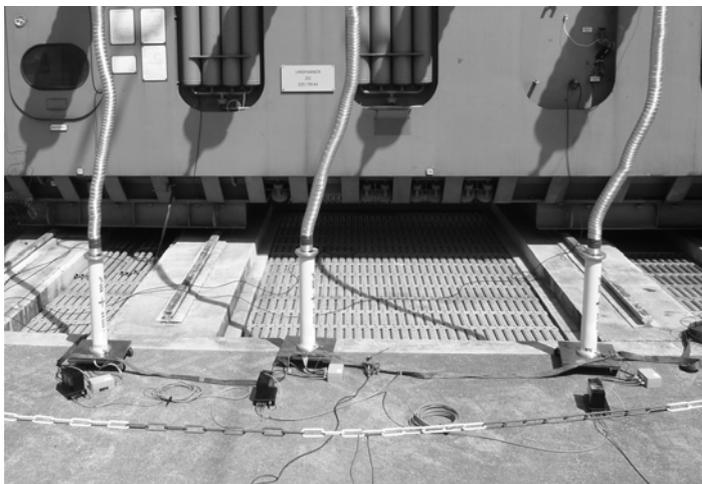
The measurements were performed on all three phases of 110 kV levels simultaneously (see Fig. 2). For these measurements three coupling capacitors of 100 pF/100 kV (AC) were available. The measurements showed partial discharge faults on phase v and w. Phase w showed the typical pattern of a void and phase v at least two partial discharge sources. One of these faults is a surface discharge and the other a void.
