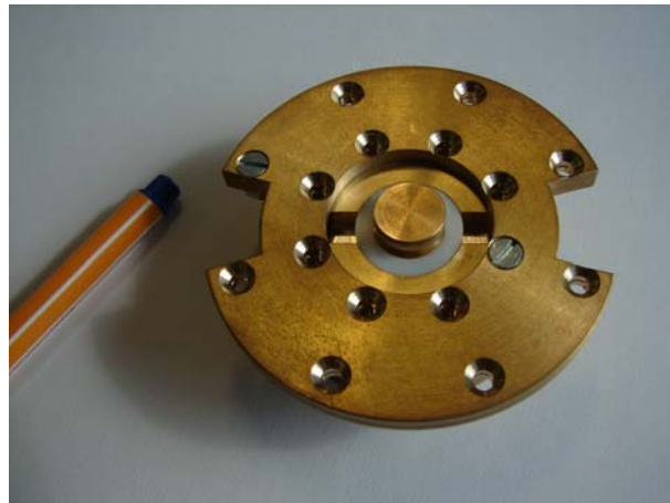
Fig. 3: Erweitertes ESD-Target zur Vermessung von SMD-Bauelementen Enhanced ESD-Target for measuring lumped Surface Mounted Devices
