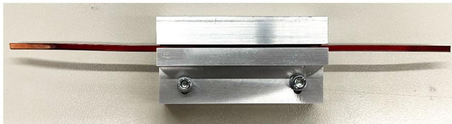
Fig. 1 Hairpin-in-slot emulation used for the degradation analysis
